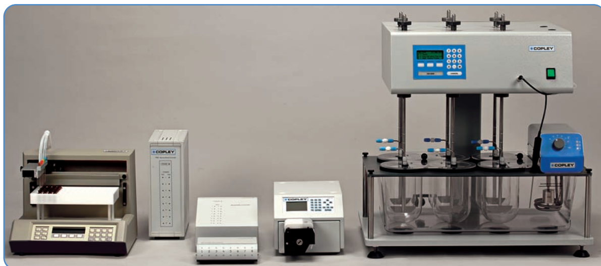
TYPICAL 'OFF-LINE' SYSTEM INCLUDING DISSOLUTION TESTER DIS 6000 AND PUMP
